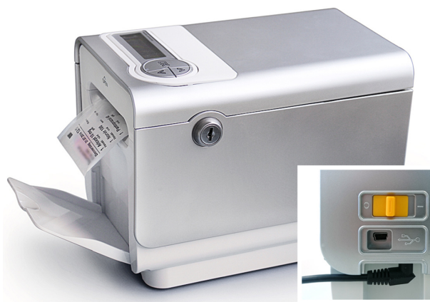
Figure 2 Remote-controlled, electronic dispenser, Medido ® , used in this study as specific electronic medication management aid for the unit-of-dose pouches.
